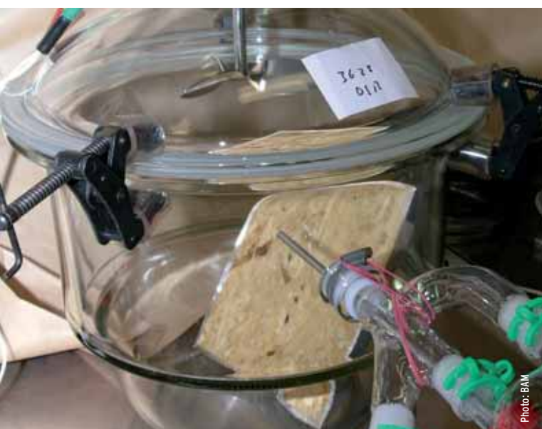
Emissions testing: Chamber with a volume of 20 litres (exicator) with a material sample consisting of a chipboard panel.
