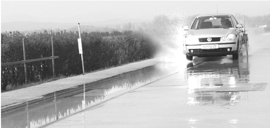
Fig.3: Test vehicle during aquaplaning measurement
