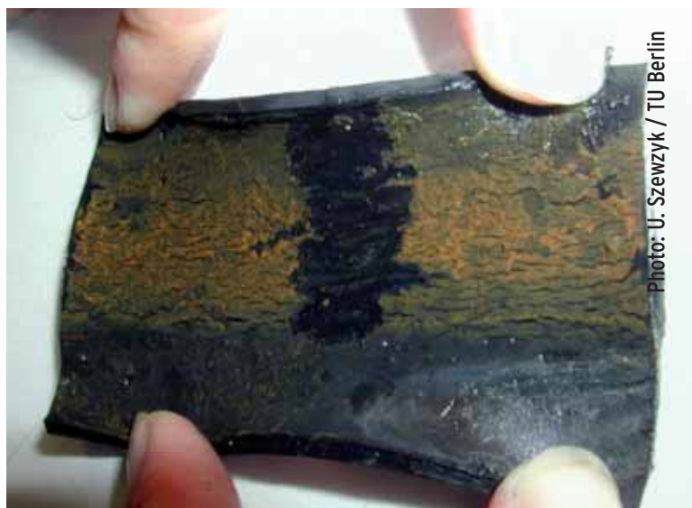
Growth of bacteria (formation of bio-film) on rubber used in drinking water systems.
