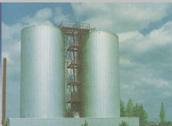
Figure 34: Bioreactor for the fermentation organically contaminated wastewater [15]
