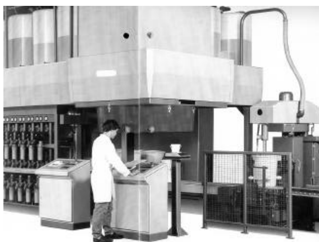
Figure 4.36: Example for an automatic printing paste preparing system, in which residual printing pastes can be reused for the formulation of new printing pastes
