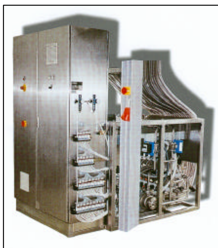
Figure 4.4: Example for the on-line preparation equipment of padding liquor for the finishing of woven and knit fabric (pictures from Mutschink GmbH, D-47918 Tönisvorst)
