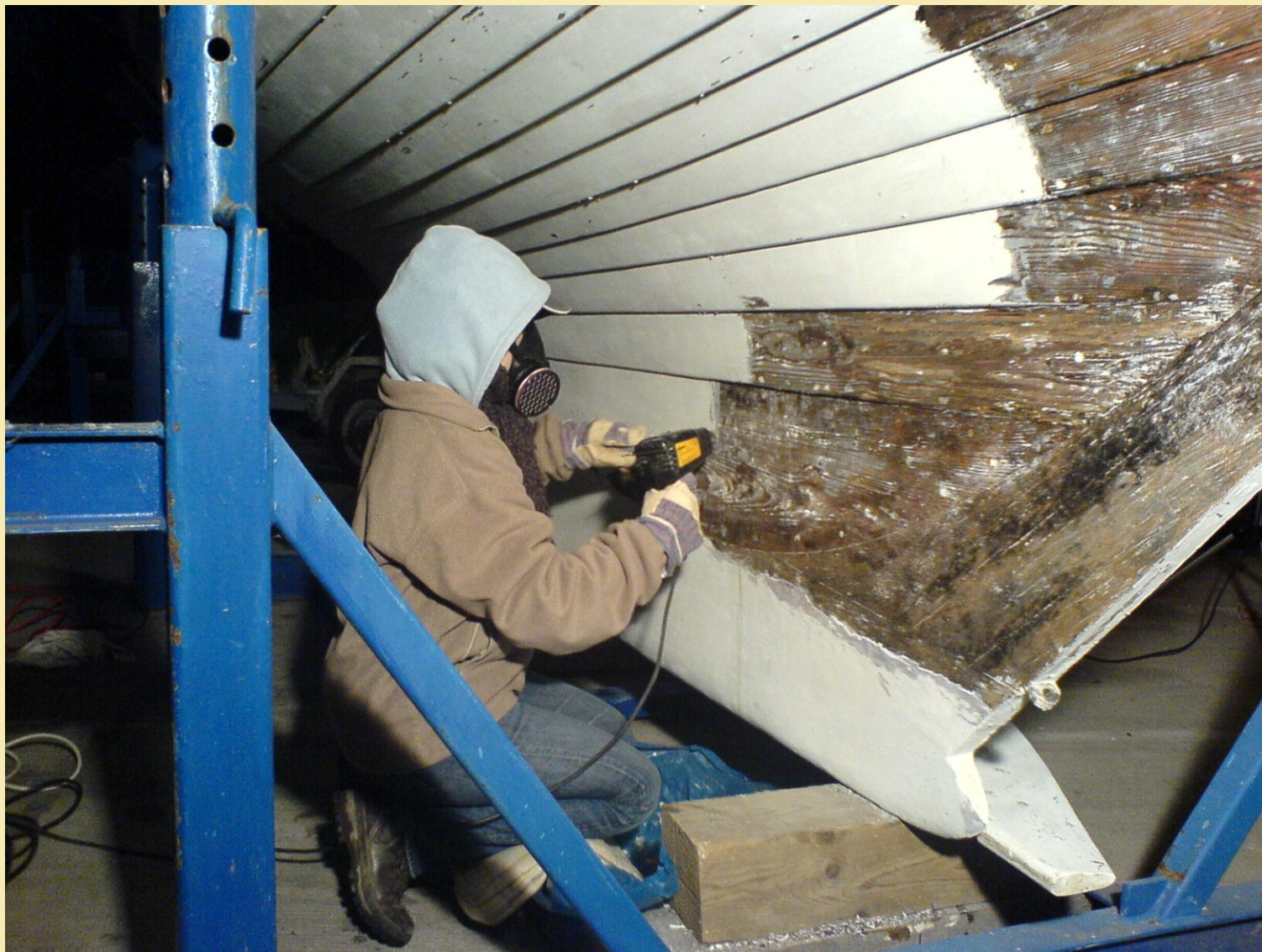
Fig. 1: Boat hull which is prepared for the use of an antifouling paint
