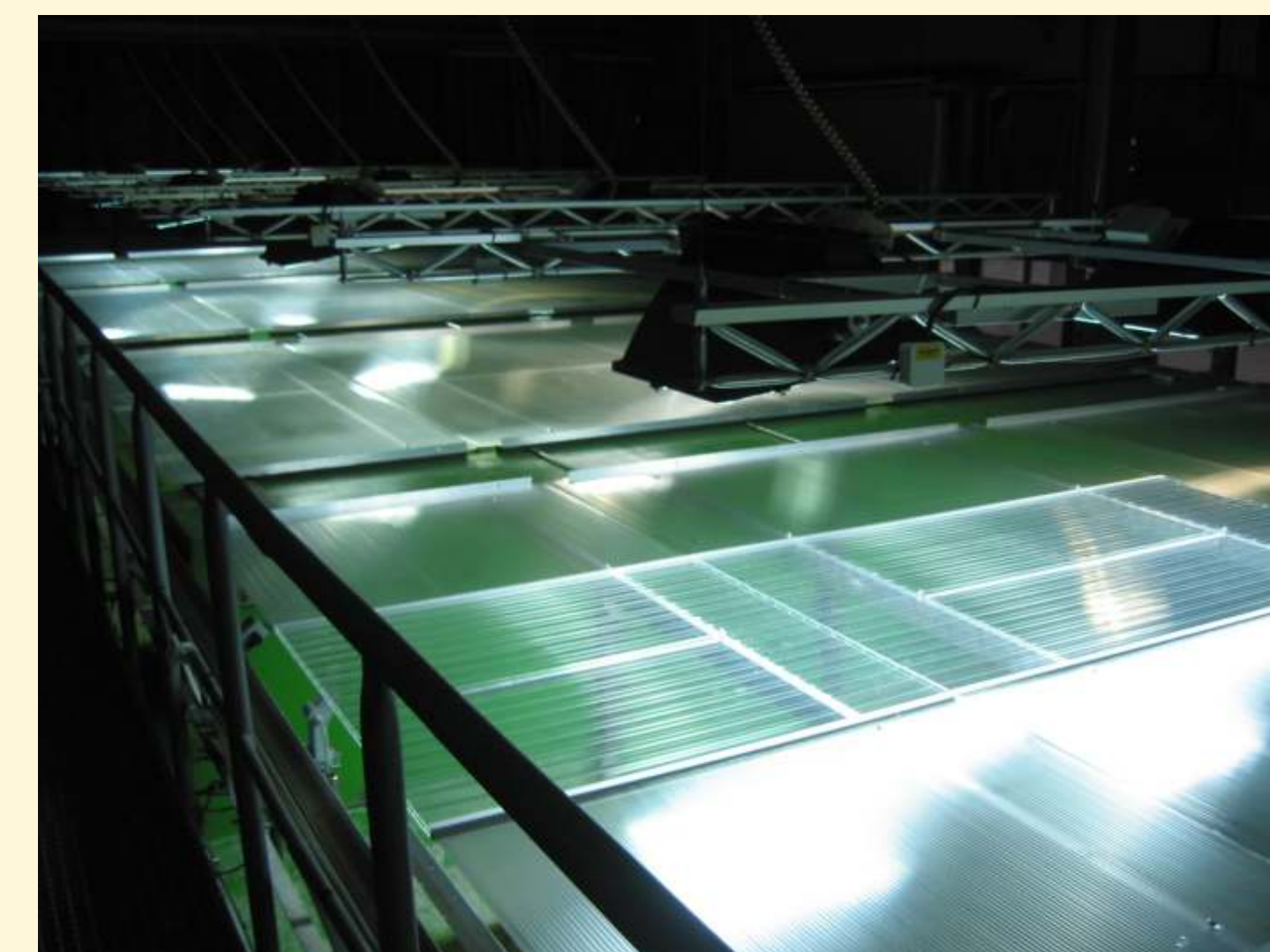
Fig. 1: Indoor pond systems (FSA) of the UBA with BFR-free plastics covers to prevent dust immission into the mesocosm system
