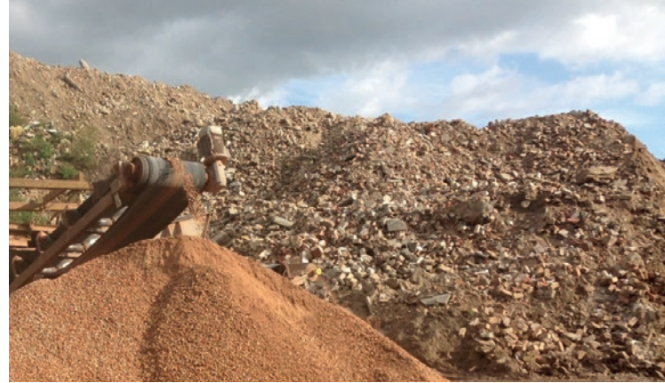
An innovative process: production of plant substrate by automated colour sorting. Automated optical colour sorting takes place in the coarse fraction. The separated red and yellow bricks are then crushed and used as granules for producing plant substrates.
