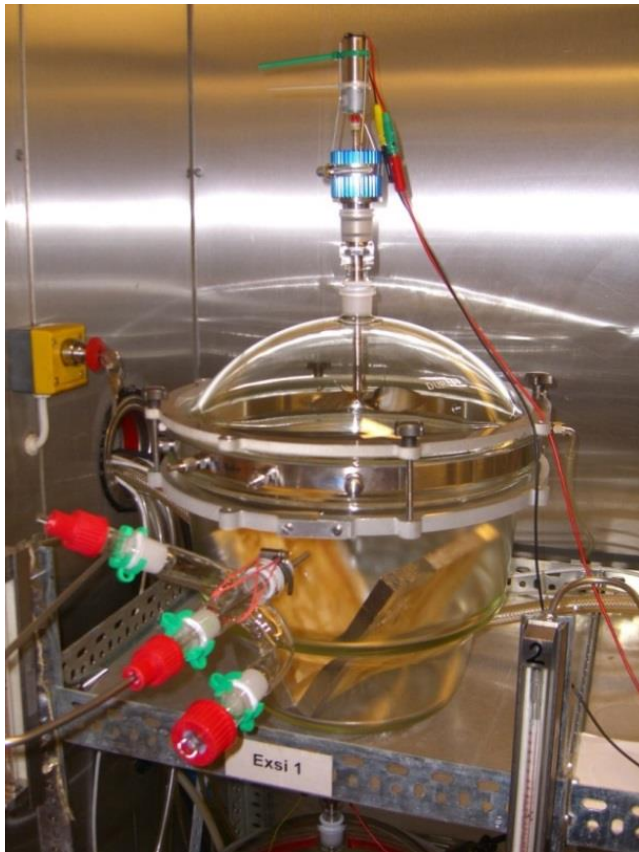
Figure 5: Testing VOC emissions in the chamber test
