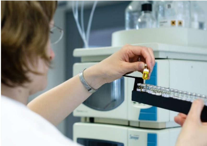
Figure 7: Indoor air samples are analysed regarding their VOC content
