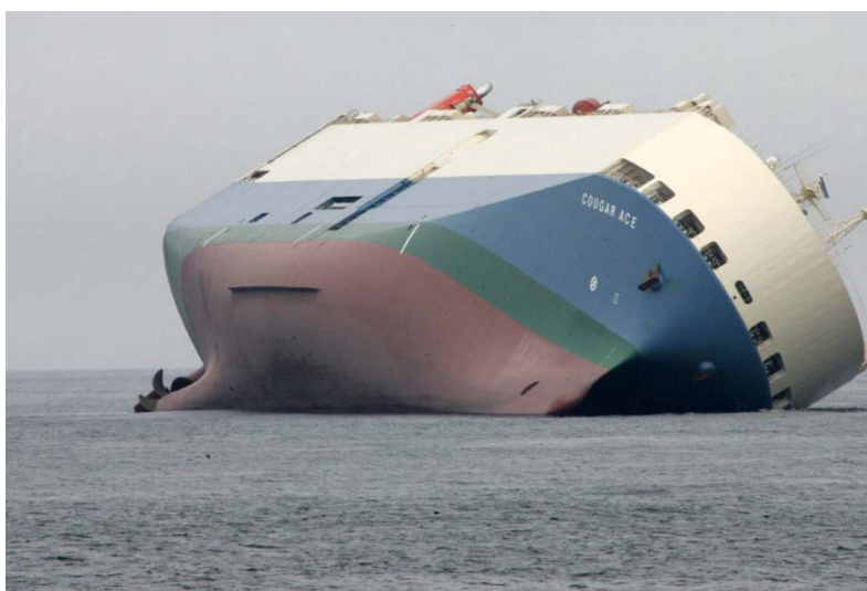
Figure 10: Loss of stability of MV Cougar Ace during open ocean exchange of ballast water on 23 July 2006 (photo: http://en.wikipedia.org/wiki/MV_Cougar_Ace ).
