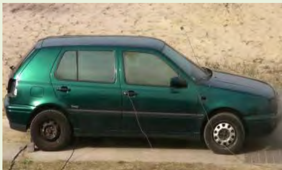
Pic. 4: Test car with windows etched by the reaction product hydrogen fluoride formed from 1234yf during a fire in the car (© UBA 2010)(14)
