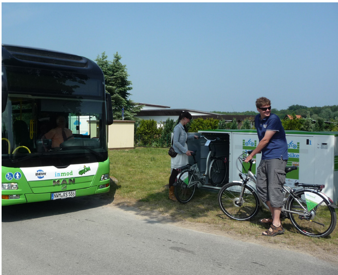
Pilotproject "INMOD – elektromobil auf dem Land" (INMOD – Electromobility in rural areas) in Mecklenburg-Vorpommer: hybrid bus with pedelec connection. Hire pedelecs are available from secure bike lockers with integrated charging stations.
