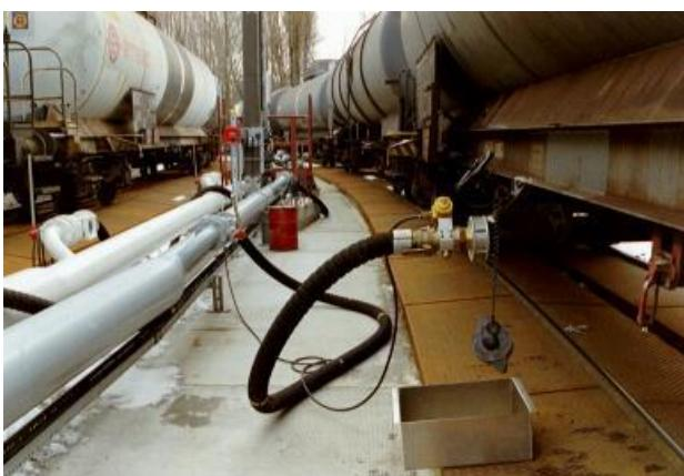
*Unloading a railway tank wagon:* Connecting pipe fitted with safety hose coupling; drips from which are collected in the mobile collecting tray.
