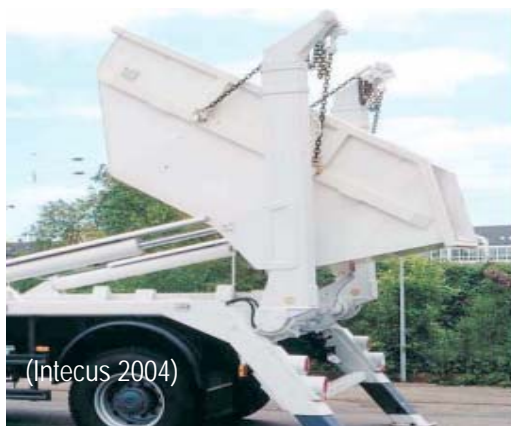
figure 6: Basic version of skip container and superstructure at the truck in tipping
