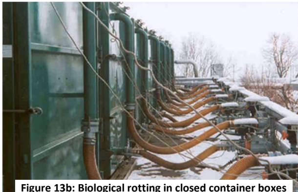
Figure 13b: Biological rotting in closed container boxes
