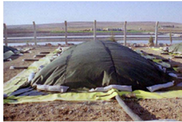
Figure 13c: Biological rotting under a semipermeable membrane
