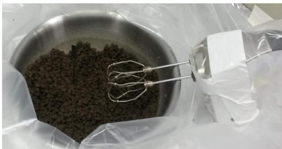
Figure 9: Photo of homogenised soil (Lufa 2.2) spiked with fenoxycarb 5
