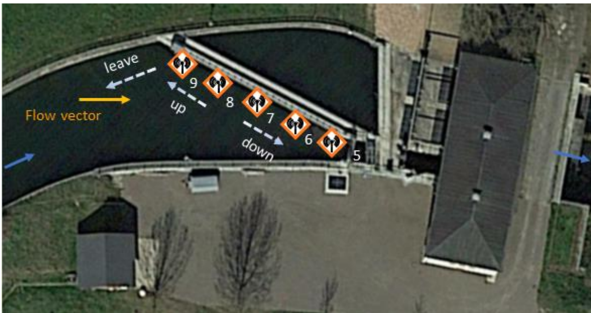
Figure 3: Arrangement of radio telemetry antennae on front of the guiding screen at the hydropower plant and illustration of the defined directions of movement.
