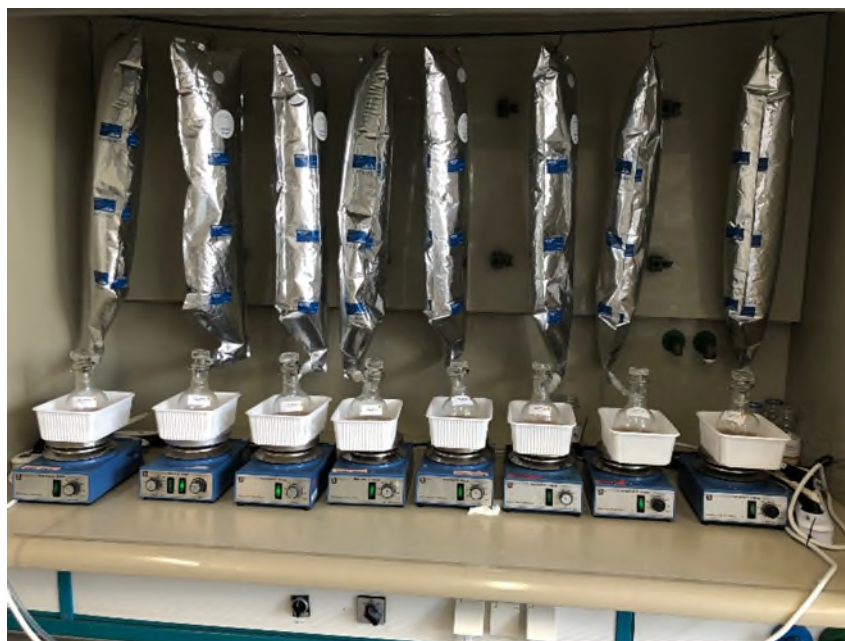
Figure 7: Schlenk flasks connected with Argon filled gas bags for silylation
